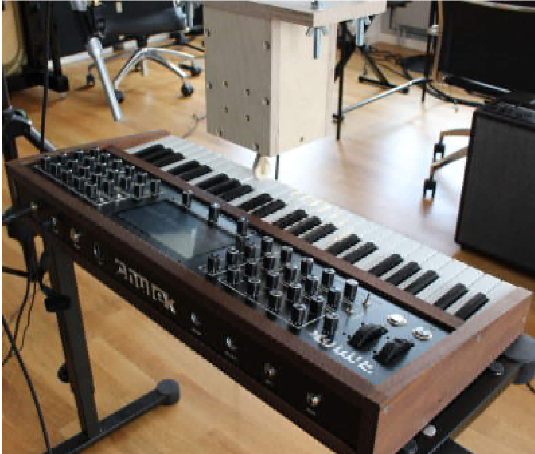
Figure 63: Synthesizer Sampling. Experiment setup showing the precise key triggering system sampling a Chulek synthesizer. The goal of this experiment was to estimate the internal velocity curves implemented by the synthesizers keyboard.
