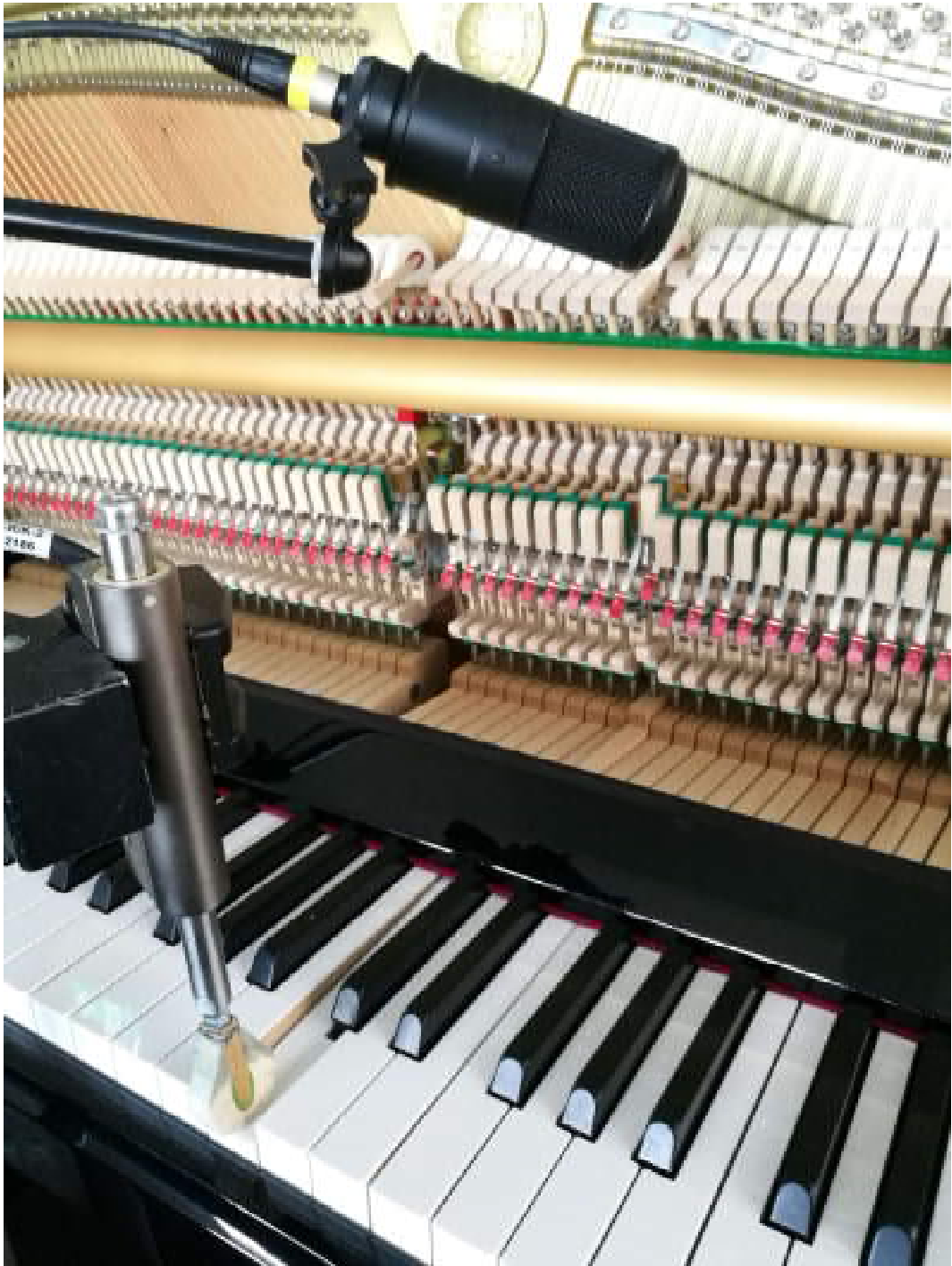
Figure 42: System Setup. The mechanical structure allows correct positioning of the actuator on the top of piano key. The microphone is installed at close to the hammer-string contact point.
