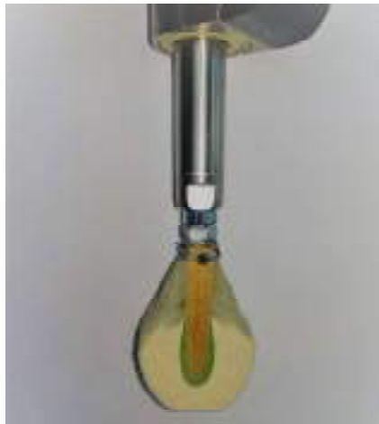
Figure 43: Hammer Felt. In order to reduce the noise produced by the contact between the actuator slider and the key, a piano hammer felt was attached to the tip of the actuator slider.
